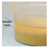
5b. Alternatively, corn samples only may be allowed to settle into layers - avoid particulates when drawing up sample
