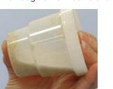
4. Cover and shake on a mechanical shaker at highest speed for 1 minute (or vigorously by hand, 2 min.)
